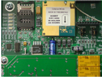
SLIDE METAL LATCH DOWN TO OPEN THE HOLDER
