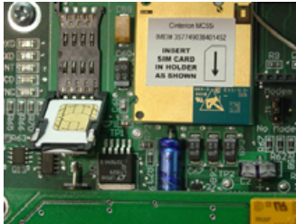
CONTACT SHOULD FACE TOWARD THE BOARD WHEN INSTALLED
