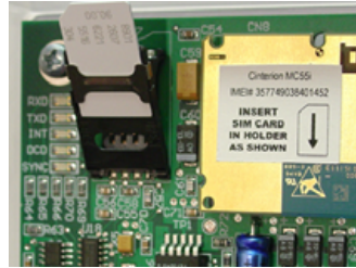
INSERT SIM CARD AS SHOWN (UPPER LEFT CORNER IS CLIPPED)
