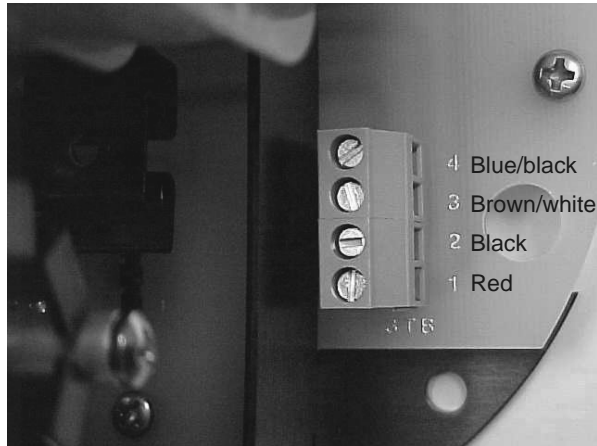
Figure 3—Terminal block 3TB on interconnect board (prewired at factory)
