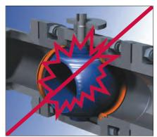
mechanically wedging out the seal slips for a positive upstream and downstream shutoff. This creates a positive, mechanical shutoff of each valve port independent of springs, system pressure or flow. In addition, the primary seals are reinforced by a secondary metal-to-metal seal, resulting in a superior, fire-safe design. Seals may be repaired with common tools while the valve is in-line, after the line has been depressurized and drained.
