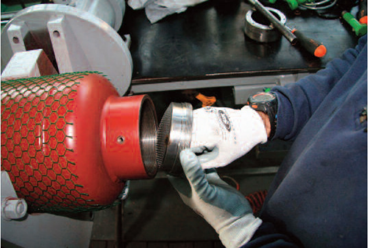
3. Install the anti-extrusion plate.
