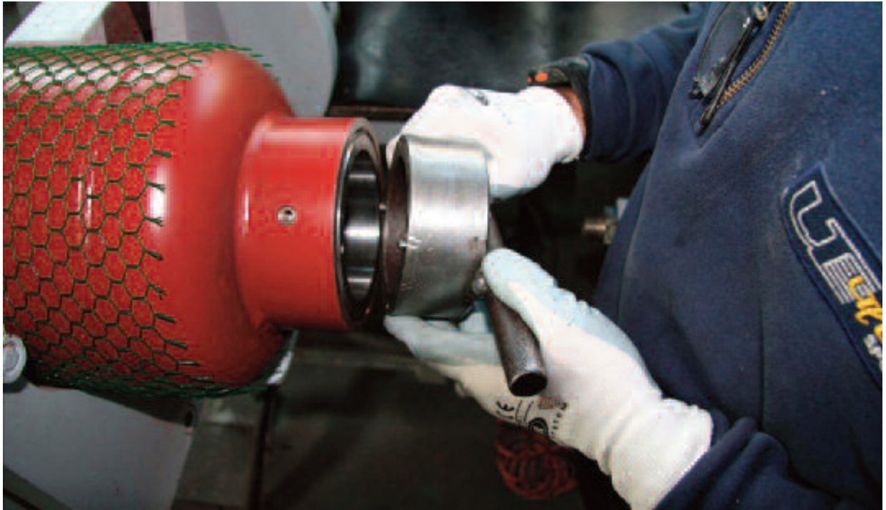
4. Using a suitable wrench, unscrew the fluid valve (anti-extrusion plate).
