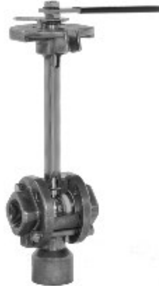
Series 21/51 Three Piece Cryogenic Diverter Valve: 1/4" through 6"; 90 or 180 degree operation; side or bottom ported; 316L stainless steel or bronze; threaded, socket weld, butt weld or flanged end connections.
