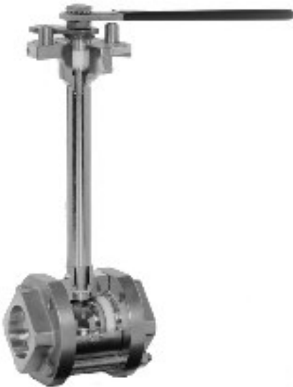
Series 2100 Three Piece Cryogenic Valve: 1/4" through 3"; 316 stainless steel or bronze; threaded, socket weld or butt weld end connections.
