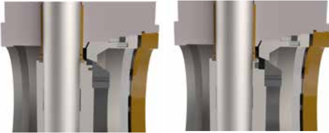
Floating seat: (new sealing)
